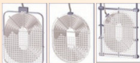
Polypropylene or polyvinyl-fluoride perforated plastic grille
